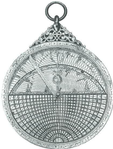
55 The front of the universal astrolabe of Ibn al-Sarrāj, dated AD 1329. This remarkable instrument not only represents the culmination of Islamic astrolabe-making, but has no equal in sophistication amongst instruments from the European Renaissance. Whereas the standard astrolabe requires a different plate for each latitude, that of Ibn al-Sarrāj has plates that serve all latitudes; indeed, the various components can be used in five different ways to solve all the problems of spherical astronomy for any latitude. IC no. 140 (Benaki Museum, Athens)
