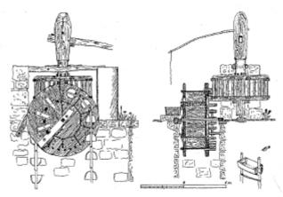
*Figure 4.* A saqiya in Ma 'arrat an-Nu 'man near Aleppo. The saqiya travelled westward and was used by the thousands in Spain until recent centuries. It reached central and south America where it was used extensively, Source. Science and Technology in Islam (STI), (UNESCO, 2002), part II, 171.
