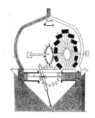
*Figure 5.* Al-Jazarî's Suction Pump. Al-Jazari described in 1206 the first suction pump. The first description of such a pump in the West is attributed to Taccola (c. 1450). Source: STI, Part II 178, or Al-Jazari's Arabic text edited by Ahmad al-Hassan (Aleppo, 1979), 465.
