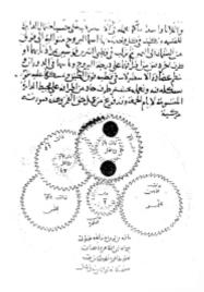
*Figure 7.* The geared calendar of al Birunî. Geared calendars and various mechanisms of the water clock were the prelude to the appearance of the mechanical clock. Source: British Library, MS OR 5593. Reproduced in Early Gearing, Science Museum (London, 1985), 34, and in Donald Hill's Studies in Medieval Islamic Technology (Ashgate-Variorum, 1998), XIV, 150.
