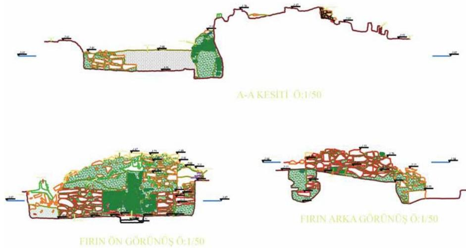
Figure 7-b. Section drawings of the iron furnace.
